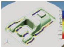
Fringe plots show the amount of uncut material on in-process models.
